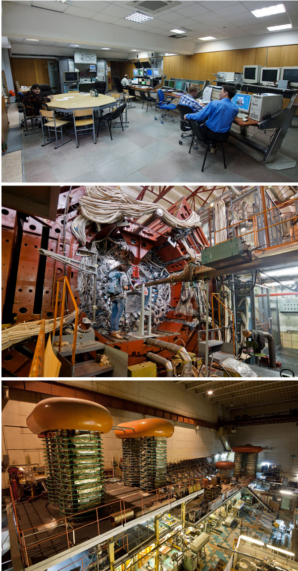
Fig. 11. The VEP-4 accelerator at the Budker Institute of Nuclear Physics. Top the control room. Middle the KEDR detector (note the standing man in the middle for scale). Bottom GOL-3 (open plasma trap) for studying high-temperature plasma. Credit: V. Makhorov.
