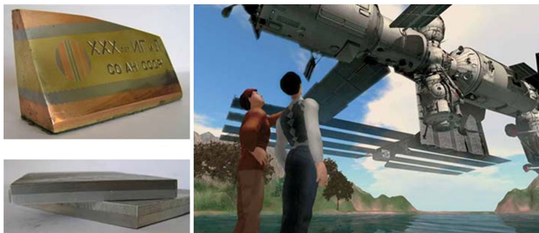
Fig. 14. Two examples of technology breakthroughs. Left pieces of copper-steel-brass ( top ), steel-duraluminium ( bottom ) welded by explosion at Lavrentyev Institute of Hydrodynamics. Right A 3-D visualization of the International Space Station (ISS) developed at the Institute of Automation and Electrometry. Sources: hydro.nsc.ru/techn1.php ; Journal Science First Hand, http://sfh_49_6-21.pdf .
